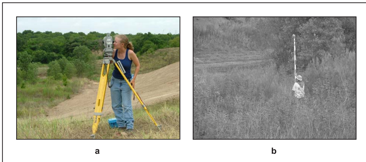
Figure 11. Topographic mapping operations and conditions in the summer of 2005: (a) EDM station and operator mapping a portion of the spillway trench; and (b) prism and operator working along north wall
