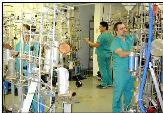
Figure 5-14. Beta Laboratory, Showing the Gas Extraction Process. (photo provided by Beta Analytic)
