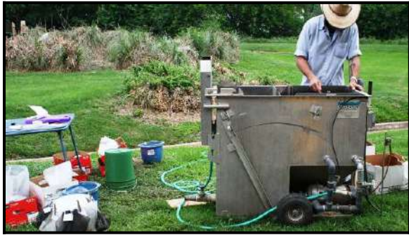
Figure 5-11. Flotation of Matrix Samples Using Dousman Flotation System.
